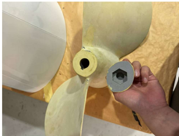
Figure 17: Applying Putty on the 3D Printed Propeller
