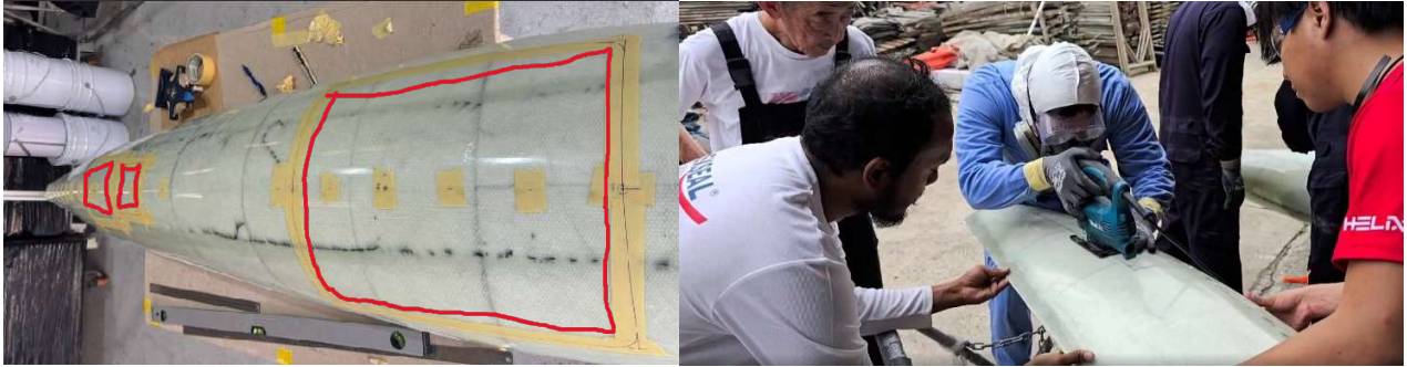
Figure 71 and 72: Measurement, Labelling, and Cutting of the Hatches
