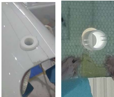
Figure 78 and 79: Strobe Light 3D Printed Mounting and Holes
