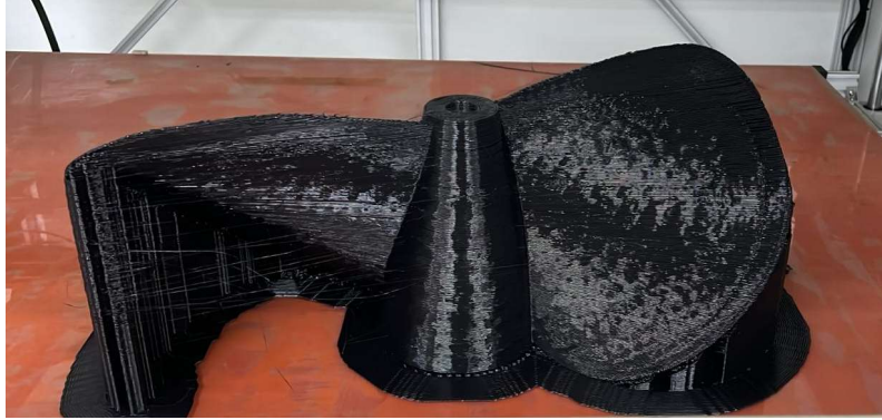
Figure 16: 3D Printing of the 2-Bladed Propeller
