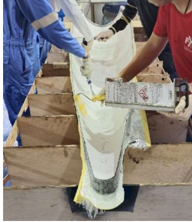
Figure 65: Applying of Resin-Hardner Mixture onto the Fiberglass sheets
