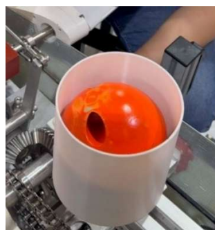
Figures 48 and 49: 3D Printed Buoy Housing with Drainage Hole
