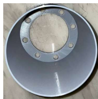
Figures 48 and 49: 3D Printed Buoy Housing with Drainage Hole
