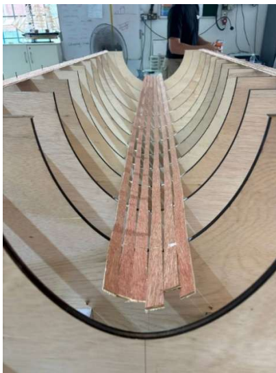
Figure 57: Skeletal Mould of the Submarine
