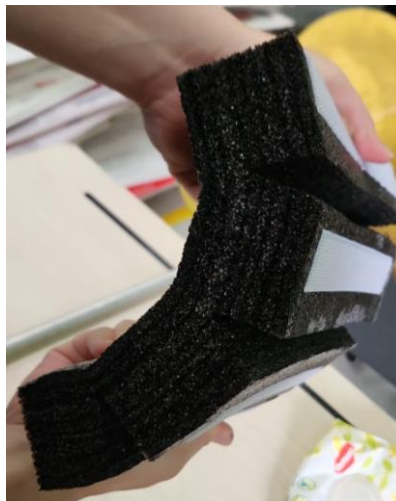
Figure 9-13 Polyethylene foam cut to match hull's internal curvature
