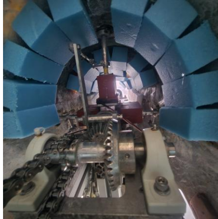
Figure 9-14 Polystyrene Foam layered inside hull
